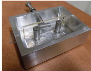
Three point continuous strain jig, as provided by Buehler.
