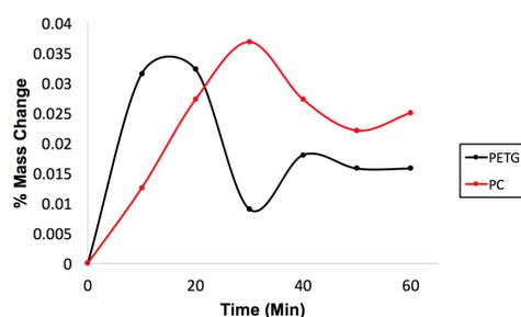
Both materials gained mass, though at only .02-.03% of total sample mass, the results are negligible. The up and down behavior shown for the PETG sample is likely a result of measurement error at small mass scales.
