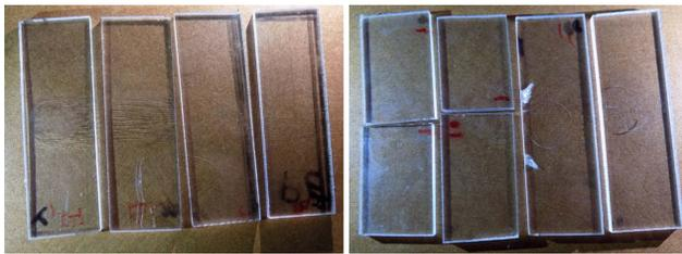
PETG (left) and PC (right) samples, displayed from left to right with decreasing strain.
