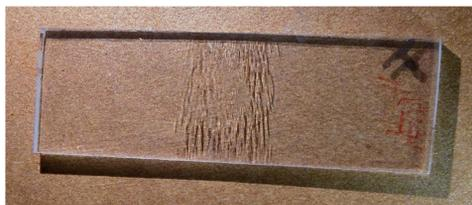
Environmental stress cracking induced in PETG during a continuous strain test soaking in Cool 3, 1 to 5 dilution, for 5 days.
