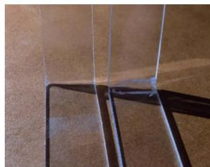
3-point bend samples before (left) and after (right) bathing in coolant for 5 days
