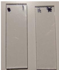
PC (left) and PETG (right) both failed to display abrasive wear from the test. Any scratches seen are a relic of the mounting mechanism, and only exists on the non-abraded side.
