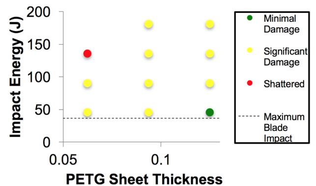
Impact strength as a function of thickness for PETG sheets.
