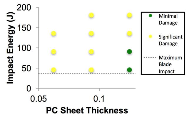
Impact strength as a function of thickness for PC sheets.
